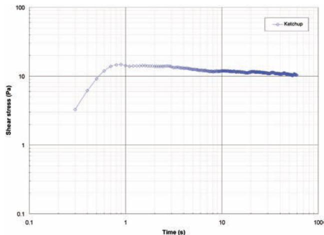
*Figure 10* Shear stress as a function of time for a commercial ketchup at 0.1  $s^{-1}$  using bob and cup, 25 mm, at 25 °C.
