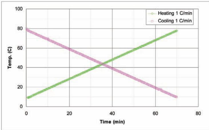
Figure 8 Temperature profiles for heating and cooling between 10 and 80 °C at a rate of 1 °C/min. The sample is 1000 cP oil using bob and cup, 25 mm,
